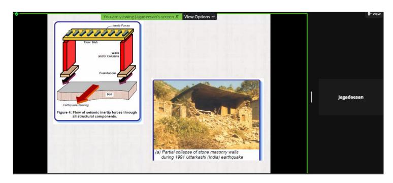
FLOW OF SEISMIC INERTIA FORCES THROUGH ALL STRUCTURAL COMPONENTS
